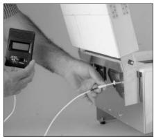
couple is positioned in the firing chamber by the correct dis-
