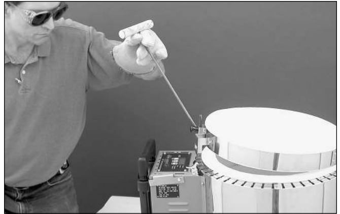
Looking at the glass during firing. Open the lid about 1". Always wear firing safety glasses when looking at the hot glass.
