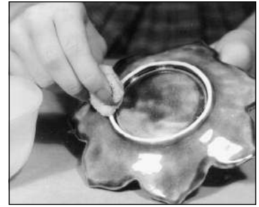
“Dry footing” means removing the glaze from the base of the piece. This eliminates the need for stilts.
