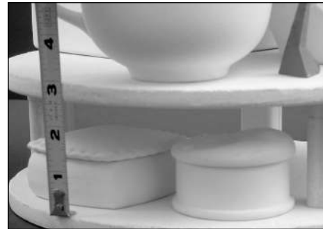
Posts in each layer should be at least 1" taller than the ware. Minimum spacing between shelves is 2 1/2" as shown above.
