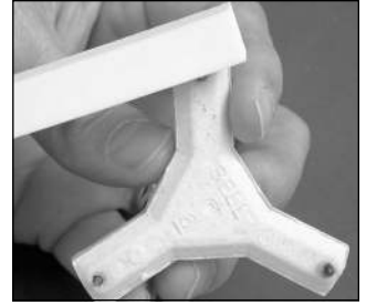
Cleaning stilt wire with a stilt stone.
