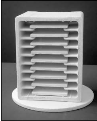
The tile setter saves space inside the kiln.
